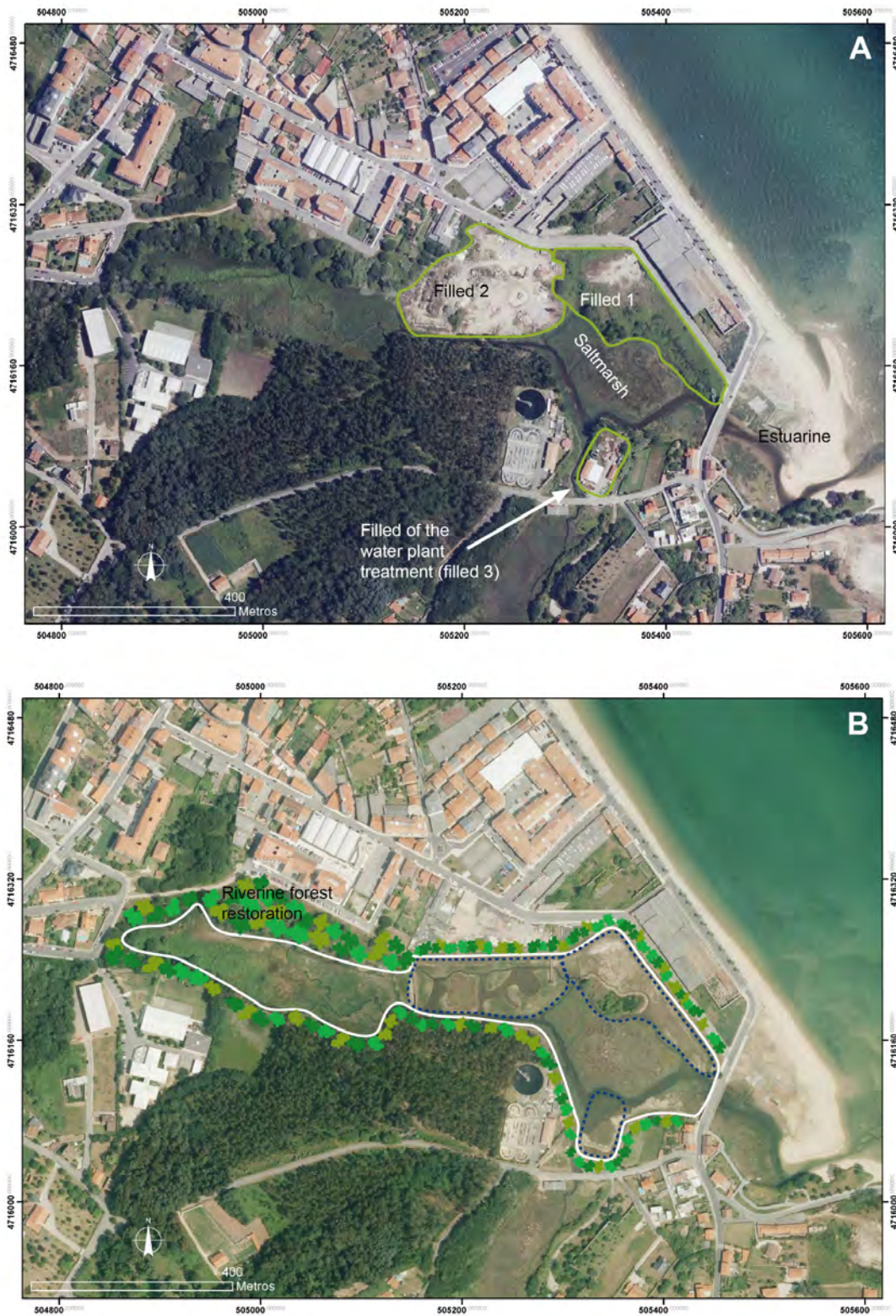
Figure 1. Aerial view of the Pobra do Caramiñal saltmarsh in 2014 (A), before the start of the interventions, and in 2017 (B), after the interventions. In the 2014 aerial photograph, sections (1), (2), and (3) indicate areas where fillings occupying more than 50% of the saltmarsh area were removed. Section (4) corresponds to the area where invasive species were removed and channels and riparian forests were restored. In the 2017 aerial photograph, sections (1), (2), and (3) correspond to newly restored saltmarsh areas.
